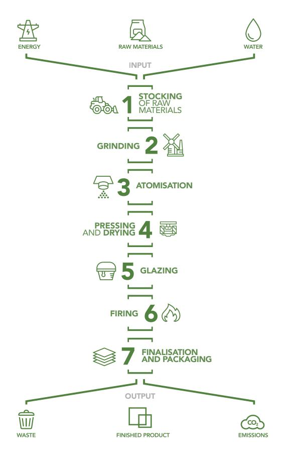
The first phase of the production process is the delivery and the stocking of the raw materials, such as clay and feldspar mixed with sand, kaolin and silicates. **Such raw materials are mined, normally in open air mines.** The production of tiles begins, therefore, from the grinding of the raw materials that are delivered to the plant and are stocked in separate, easily identifiable boxes in covered areas.
